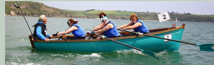
**The Bursledon Gig** harks back to the days when every waterman, boatyard worker and fisherman on the Hamble river (UK) would row to work. The latest boats are based on a GRP version of an oyster dredging punt, sea-worthy, stable, sturdy but easily rowed. The gig is 15'4" long with a beam of 5'4". It can be rowed by 1, 2, 3, 4 or 6 rowers, with or without a cox.
