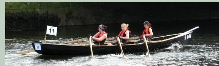
**A three-hand racing currach:** of a lighter build than their working counterparts, racing currachs are more streamlined and faster. Like all the currachs in this race, the oars are fixed to the boat using a pin (wooden or metal), which goes through a block on the oar. This means that the oars cannot be feathered (turned sideways when moving through air). The oar blades are very narrow compared to other kinds of rowing boats.
