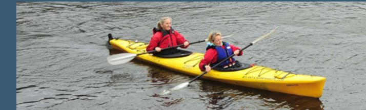
The types of **kayak and canoe** seen in the race include touring sea kayaks, racing kayaks, sit-on-top kayaks, surf skis and Canadian canoes. A touring sea kayak (seen here) is a long relatively wide and stable kayak with a covered deck (sit-inside) with good hull volume to bounce on top of waves.
