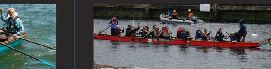
**The Bursledon Gig** harks back to the days when every waterman, boatyard worker and fisherman on the Hamble river (UK) would row to work. The latest boats are based on a GRP version of an oyster dredging punt, sea-worthy, stable, sturdy but easily rowed. The gig is 15'4" long with a beam of 5'4". It can be rowed by 1, 2, 3, 4 or 6 rowers, with or without a cox.
